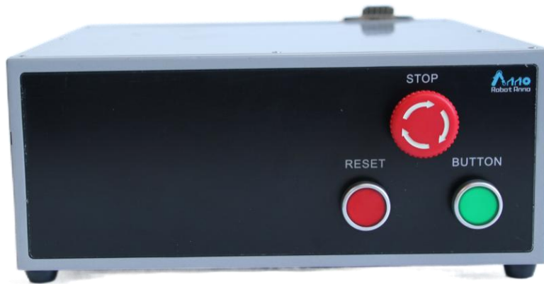
- Figure 22 PROBOT G602 Appearance of the electronic control box of the robot arm
