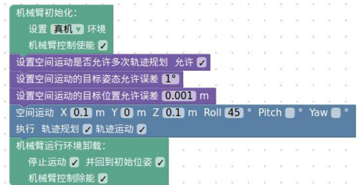
- Figure 75 Blockly Graphical Programming Example - Cartesian Motion
