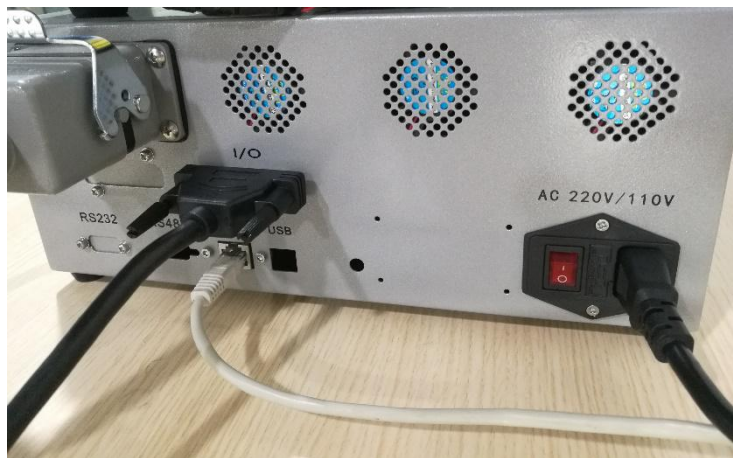
Control box power connection physical map
